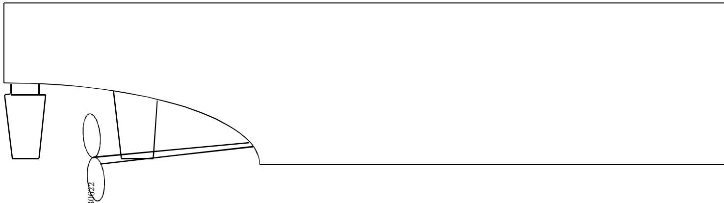
Conventional propeller/stern arrangement with horizontal shaft, strut, propeller, and rudder (not to scale)
